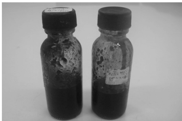
Figure 3 Bio-oil from Water-cooled condenser and ESP
