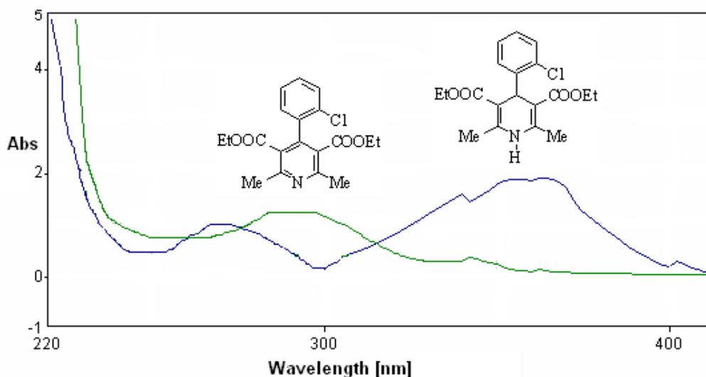
**Figure 2.** UV spectra of diethyl 2,6-dimethyl-4-(4-chlorophenyl)-1,4-dihydropyridine-3,5-dicarboxylate (**5d**) and its photoproduct (**6**)
