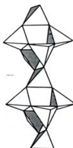
Figure 6 The tetrahedra linked together to create a three-dimensional structure Source: Dyer (1988)
