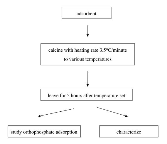
**Figure 8** The scheme of natural zeolite calcination
