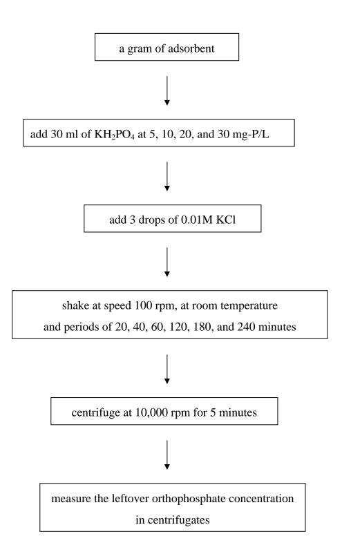
Figure 9 The scheme of orthophosphate adsorption procedure
