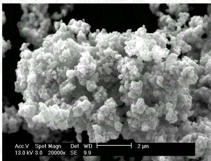
Figure 23 SEM image of N-S co-doped TiO 2 using titanium(IV) tetraisopropoxide as a titania precursor calcined at 600°C.
