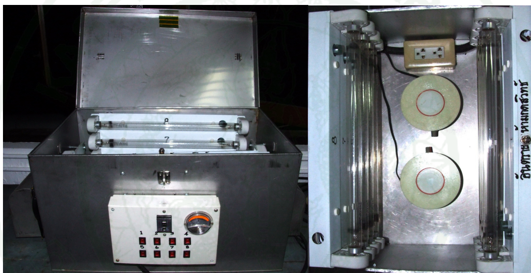
Figure 7 The image of photoreactor contained UV-lamps and magnetic stirrers.
