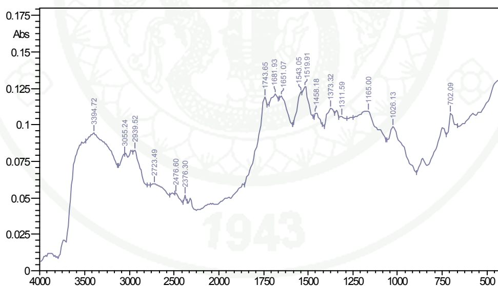
Appendix Figure A6 FT-IR spectrum of \gamma -PGA-graft-L-PAE with grafting degree of 49%.
