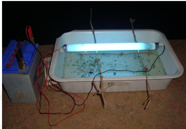
Figure 5 Light trap for collection of adult specimens of Trichoptera at Mae Tao and Mae Ku watersheds, Mae Sot District, Tak Province, northern part of Thailand.
