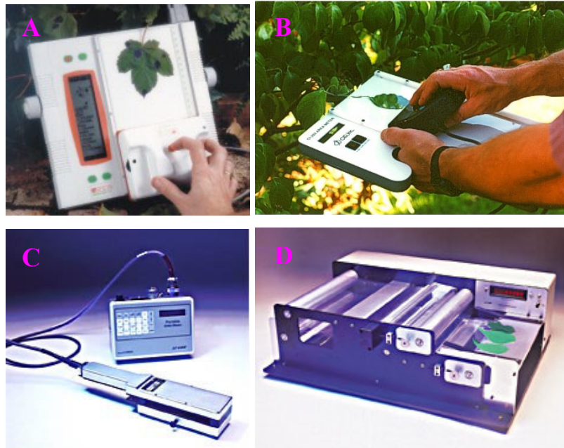
Figure 3 Leaf area meter A) AM-3000 (ADC BioScientific Ltd); B) CI-202 (CID, Inc.); C) LI-3000A (LI-COR Inc.); D) LI-3100 (LI-COR Inc.)
