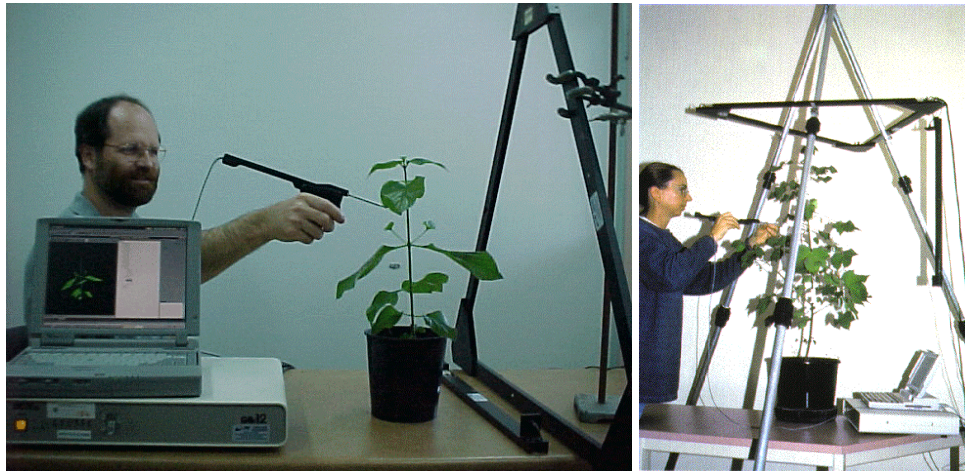
Figure 5 Measurement of plant architecture using ultrasonic digitiser
