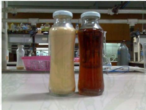
**Figure 27** Palm fatty acid distillate at; room temperature (left); higher than 50 °C (right)
