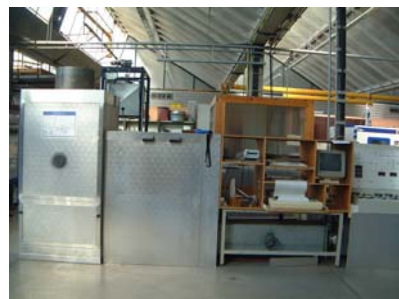
Figure 16 Schematic diagram of the drying apparatus (Hohenheim Type, the University of Hohenheim, Stuttgart, Germany).
