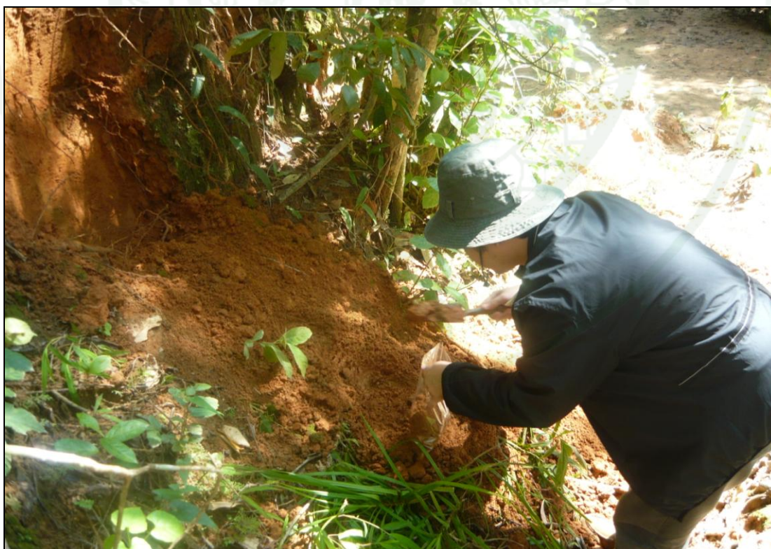
Appendix Figure 4 Disturbed soil sampling for testing in laboratory.
