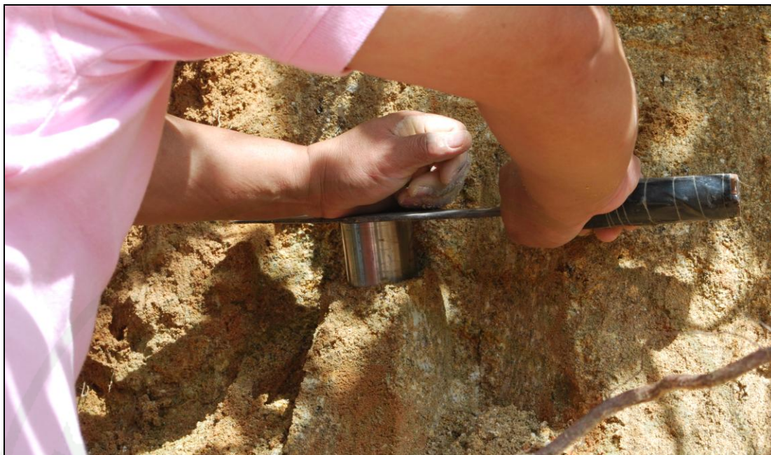
Appendix Figure 3 Undisturbed soil sampling for testing in laboratory.
