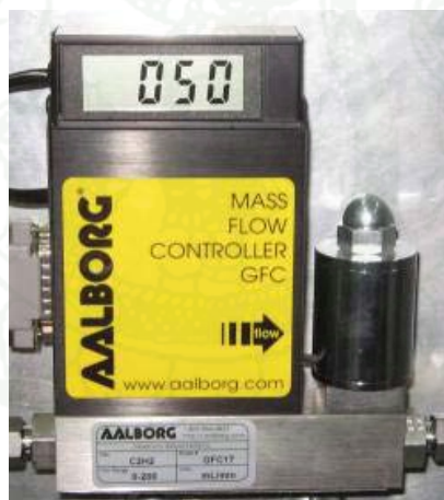
Figure 16 Mass flow controller (GFC117 Model, Aalborg).
