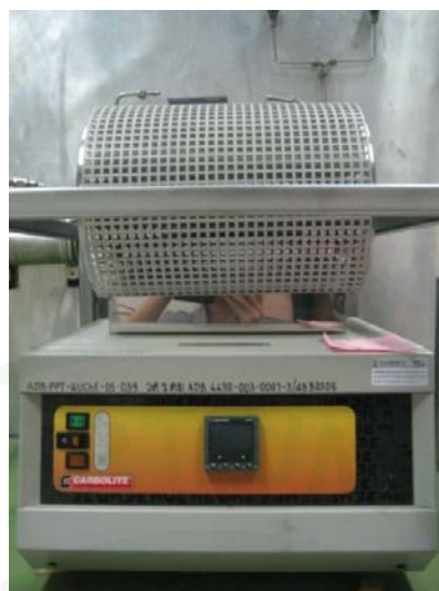
Figure 17 Tube furnace (MTF 12/38/250 Model, Carbolite).
