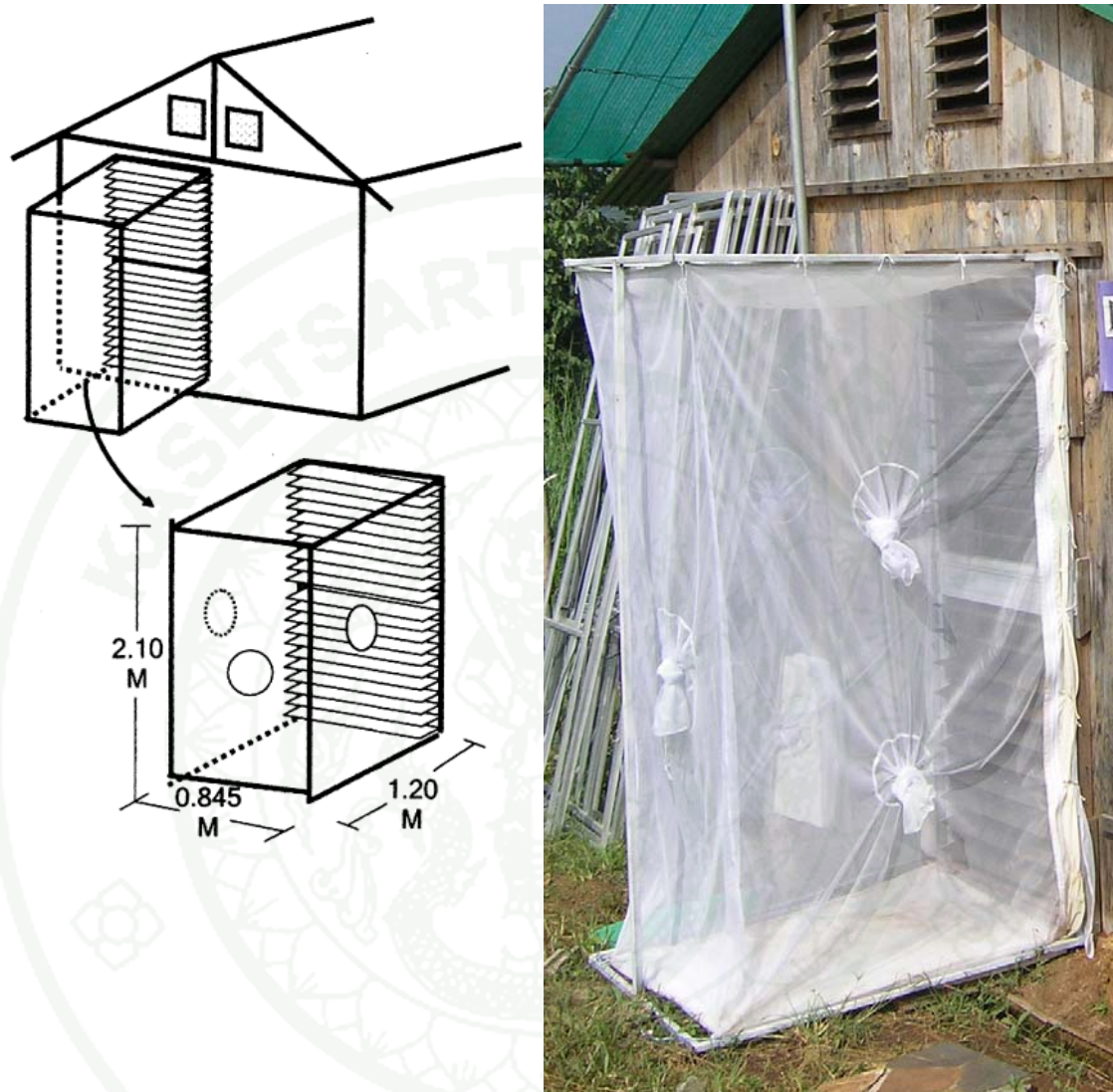
Figure 11 Door trap fixed to the door opening.
