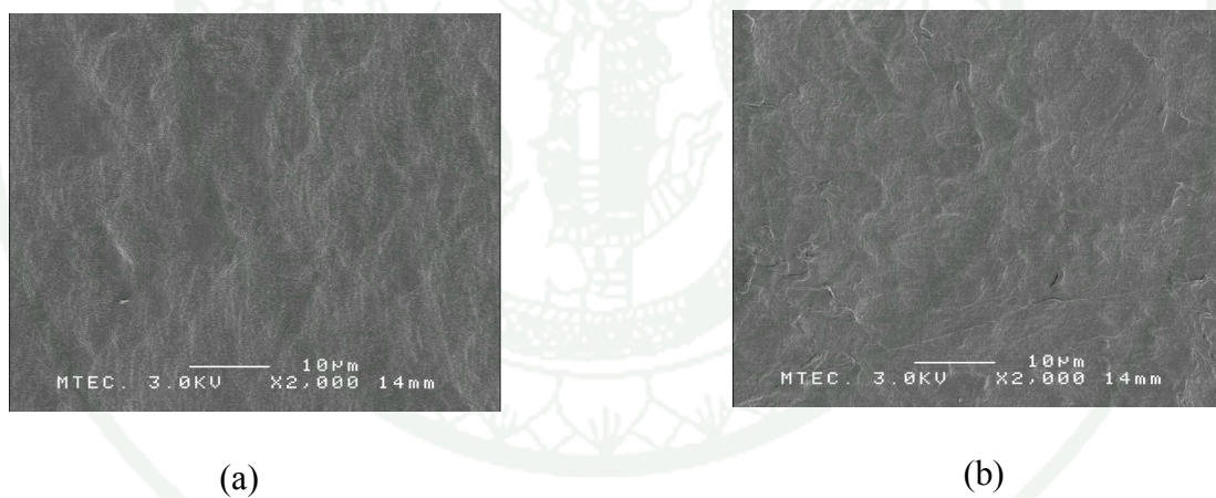
Figure 66 SEM micrographs of surface of PE before (a) and after biodegradation testing (b) after 90 days.
