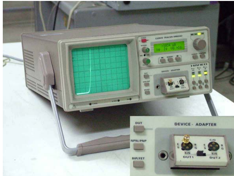
Appendix figure B5 Measurement of Diode Characteristic with HM6042
