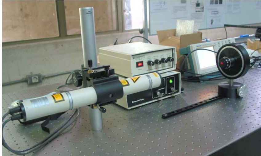
Figure 35 SP117 laser head is aligned direct into the OSA to evaluate the Etalon cavity expansion co-efficient
