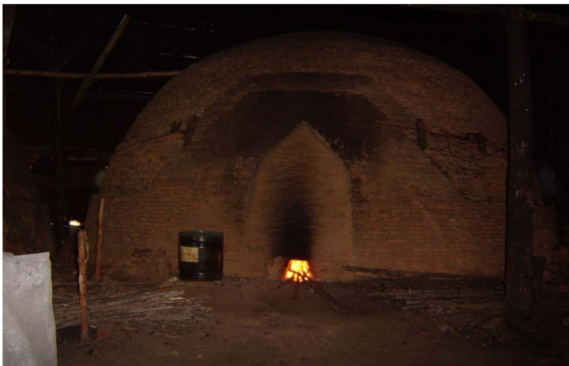
Figure 23 Dome-shaped brick beehive charcoal kiln under Nipa roof in Yeesarn Sub-district, Samut Songkram Province.
