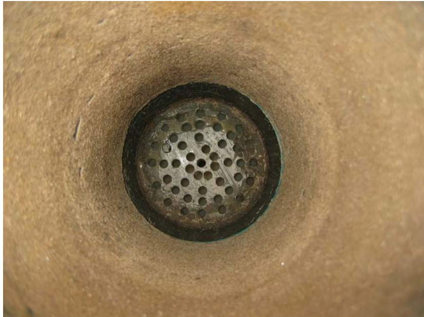
Appendix Figure E10 Sand layer on inside column wall
