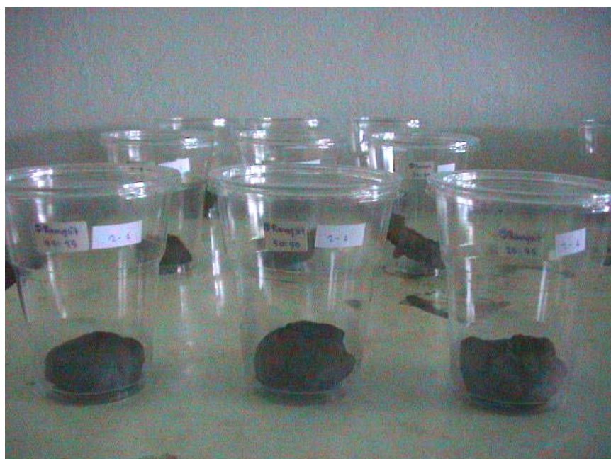
Appendix Figure E5 Soil-sludge amendment incubation
