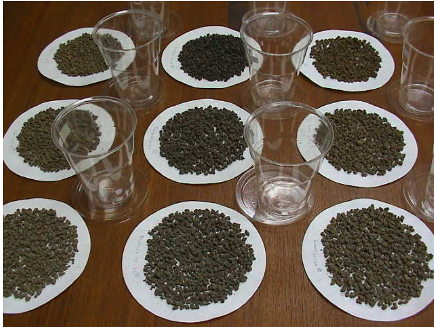
Appendix Figure E6 Air-drying of soil-sludge amendment
