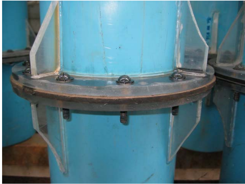
Appendix Figure E8 Column separator to ease column cleaning
