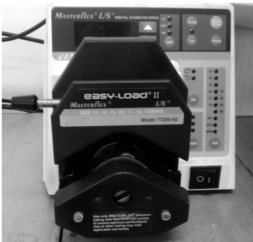
Appendix Figure C3 Peristaltic pumps
