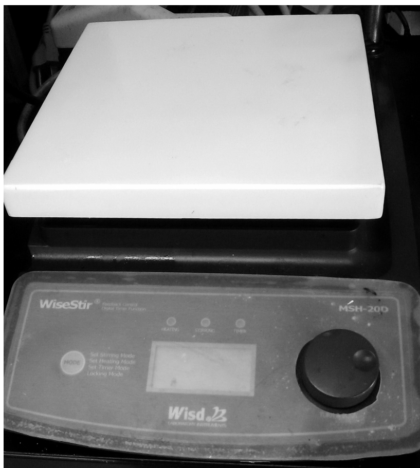
Appendix Figure C4 Hotplate magnetic stirrer
