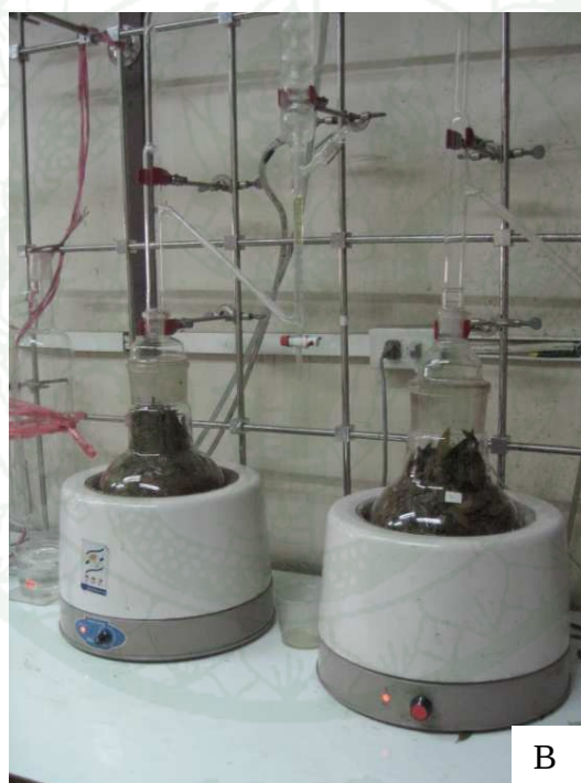
Figure 8 A) The rhizomes were cut into small pieces and B) a Clevenger-type apparatus
