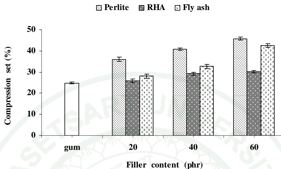
Figure 32 Compression set of the NR vulcanizates filled with various filler content.
