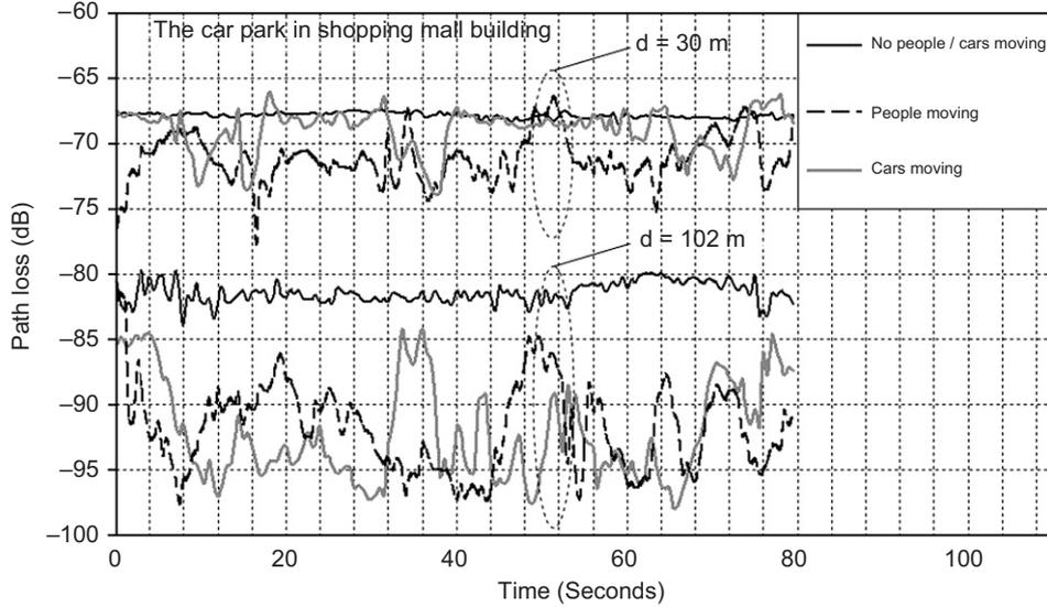
Fig. 7. The fading path loss measurement.
