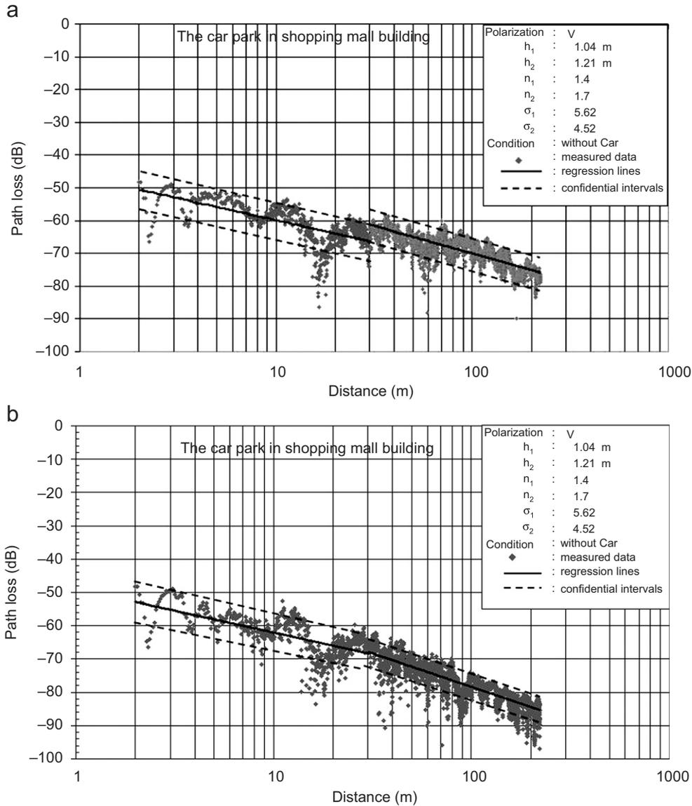
**Fig. 6.** The path loss measurement and the regression lines in the car park inside the shopping mall building. (a) no cars moving (b) with cars moving.
