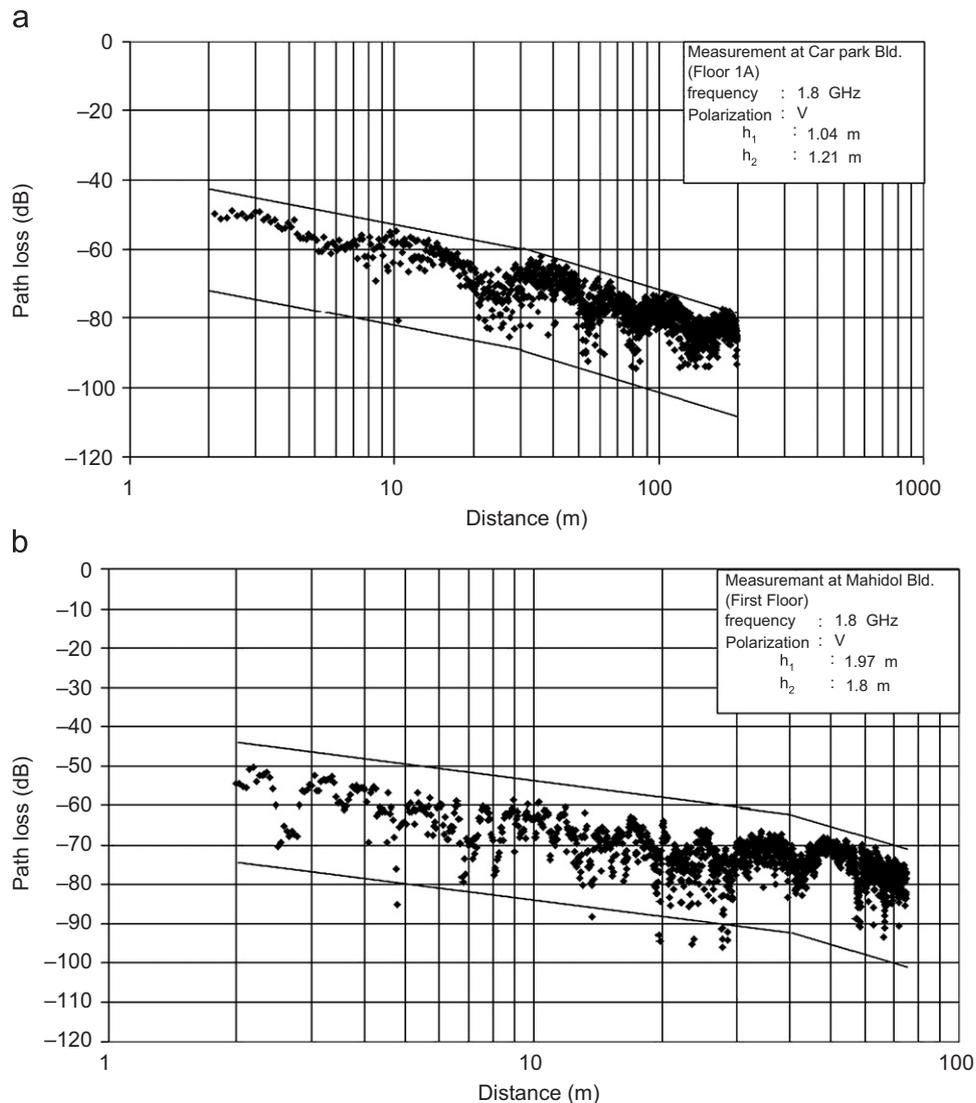
**Fig. 9.** The path loss measurement and the proposed models in different building. (a) Car park inside the shopping mall building (b) Concrete school building.
