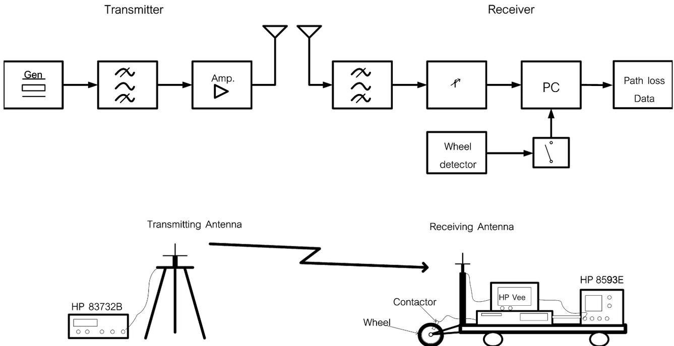
Fig. 1. Measurement system.
