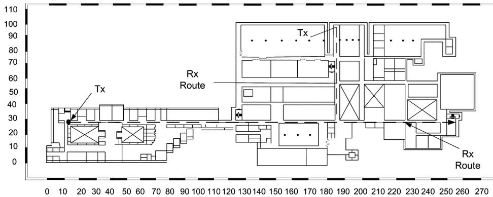
Fig. 2. Measurement location of the concrete school building.
