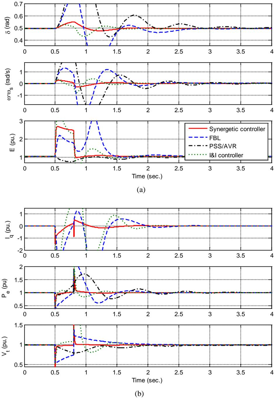
**Figure 3** Temporary fault case: Time histories of (a) Power angle ( $\delta$ ), relative speed ( $\omega - \omega_s$ ) and transient voltage ( $E$ ), (b) STATCOM current ( $I_q$ ), Active power ( $P_e$ ) and terminal voltage ( $V_t$ ). (Solid: Synergetic controller, Dashed: FBL controller, Dashdotted: PSS/AVR, Dotted: I&I controller)
