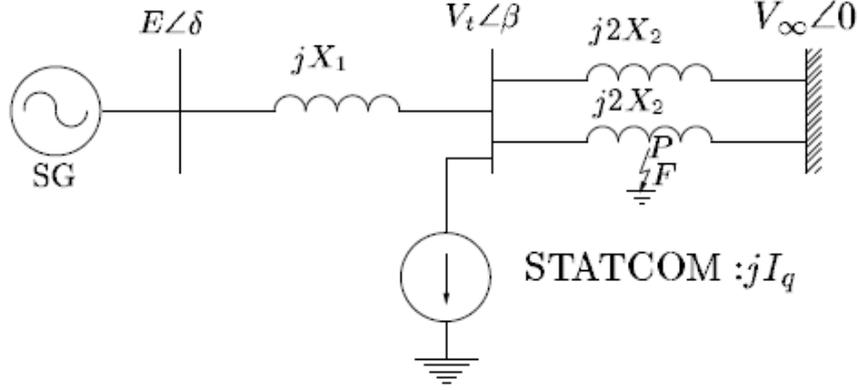
Figure 2 A single line diagram of SMIB
