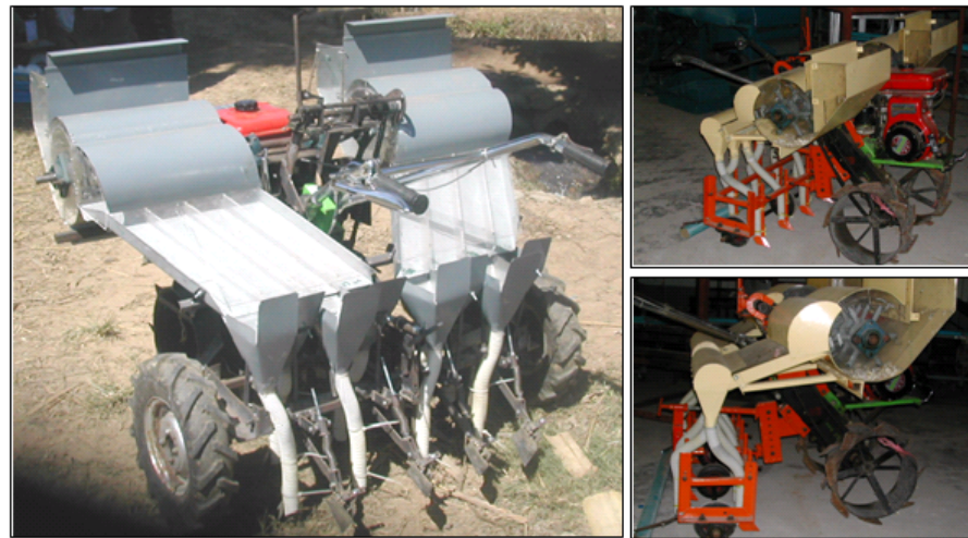
Figure 8 the 8 rows garlic planter installed with 5 HP engine power tiller
