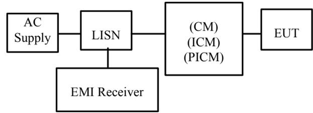
Figure 6 test setup of conducted EMI measurement
