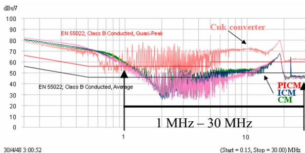
Figure 8 experimental result of conducted EMI
