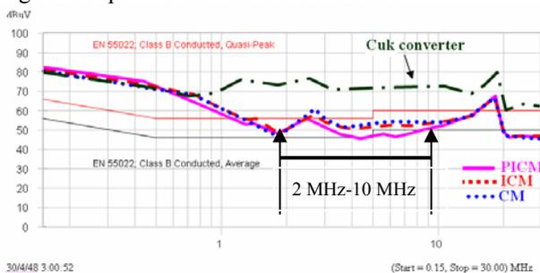
Figure 9 envelope of conducted EMI for four cases
