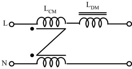
Figure 3 the equivalent circuit of integrated common mode choke (ICM) [4]
