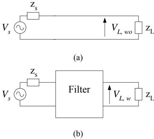
Figure 5 the definition of the Insertion loss of filter
