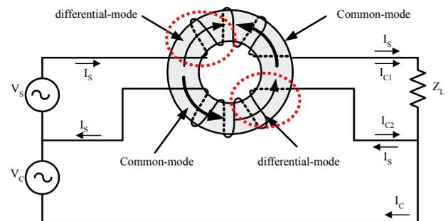
Figure 1 the flux direction of common-mode choke
