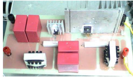
Fig. 6. Ćuk converter for case 1
