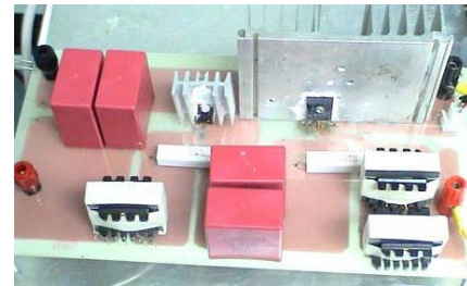
Fig. 8. Ćuk converter for case 2
