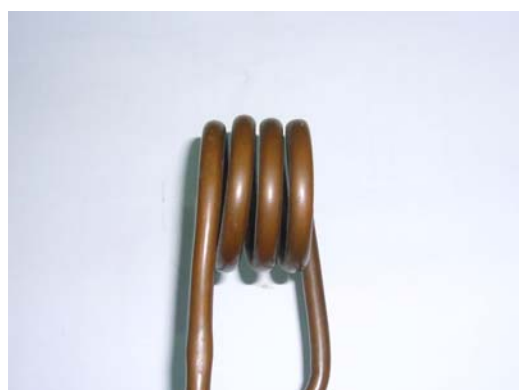
working coil = 4 turns
