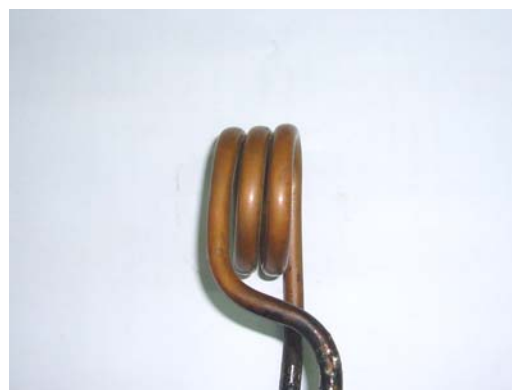
working coil = 3 turns
