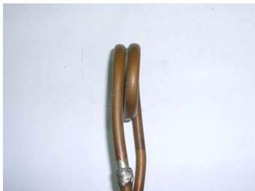
working coil = 2 turns
