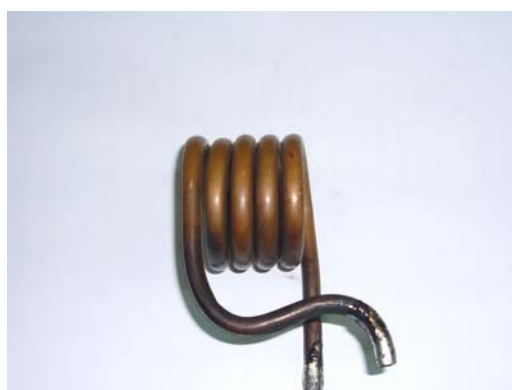
working coil = 5 turns
