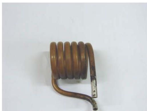
working coil = 6 turns
