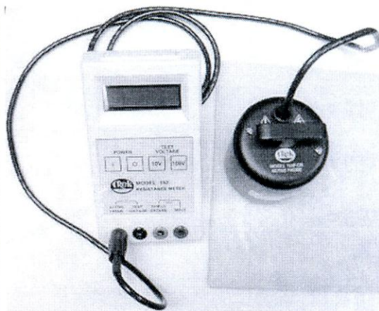
Figure 4: Surface resistivity measurement setup.
