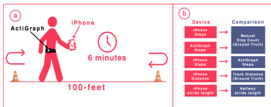
Figure 2.16 Consenting patients performed a 6MWT along a pre-measured 100-foot course with an iPhone in one hand and an ActiGraph GT9X attached at the waistband on the right hip (150)
