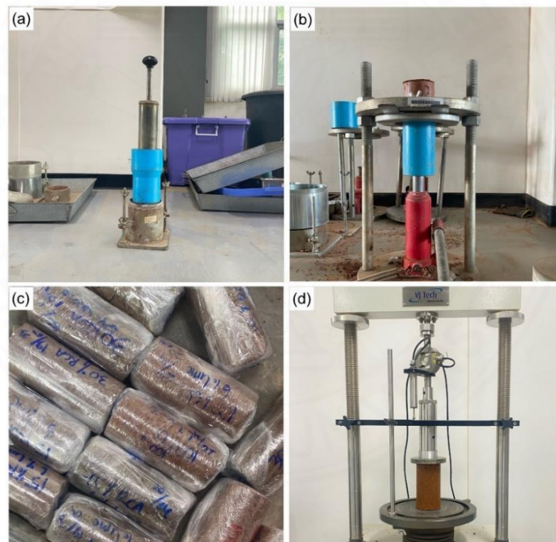
Figure 3.12 UCS test: (a) compaction of soil in a PVC mold, (b) extrusion of the sample, (c) wrapping the samples for curing, and (d) conducting the UCS test.
