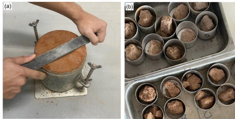
Figure 3.11 Compaction test: (a) leveling the surface of the soil sample and (b) soil samples after oven drying to determine water content.
