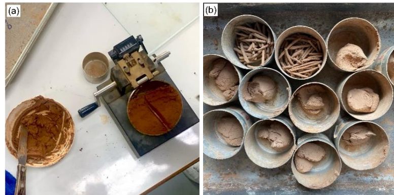
Figure 3.9 Atterberg limit equipment: (a) Casagrande device for liquid limit determination and (b) soil samples after oven drying.
