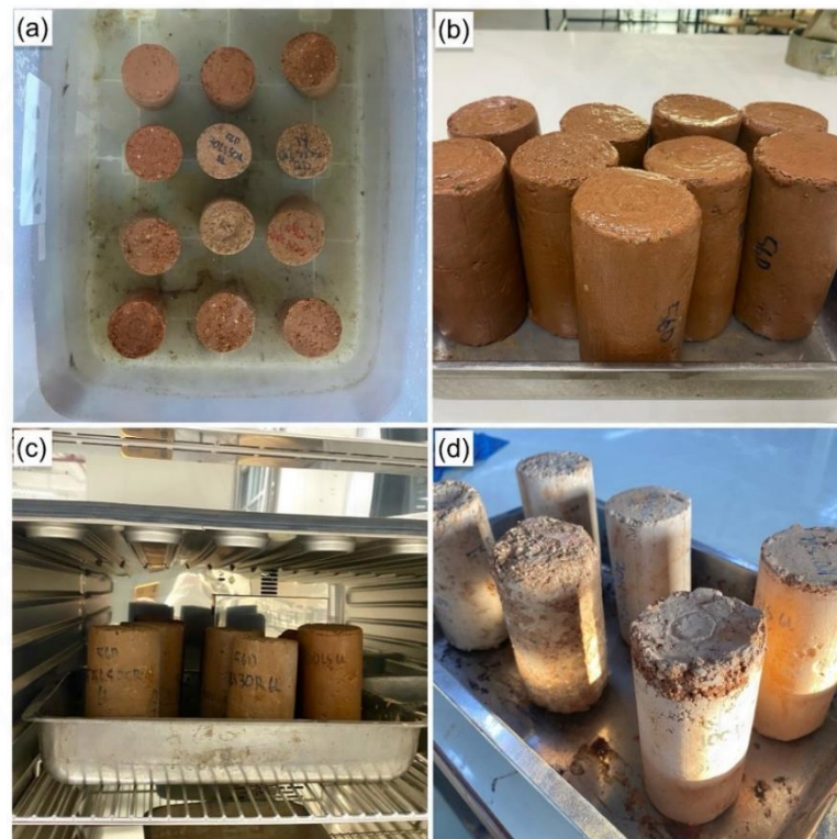
Figure 3.13 UCS under wetting and drying: (a) samples under wetting conditions, (b) samples after soaking for 5 hours, (c) samples during drying conditions, and (d) samples after oven drying for 2 days.
