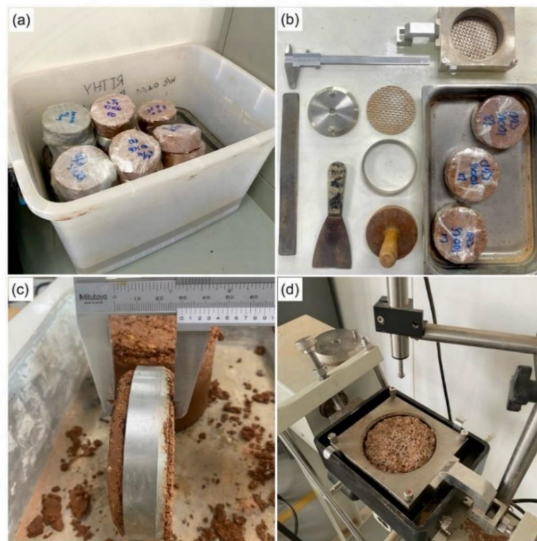
Figure 3.15 Direct shears: (a) curing conditions (b) sample preparation, (c) sample measurement, and (d) shear box set up.
