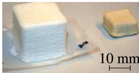
Figure 2.12 Evolution of printed object after drying at 25 °C Source: Reproduced from Klar et al. (2019).
