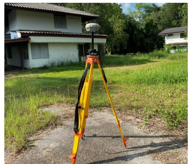
Figure 9 GNSS receiver setup at point BM4
