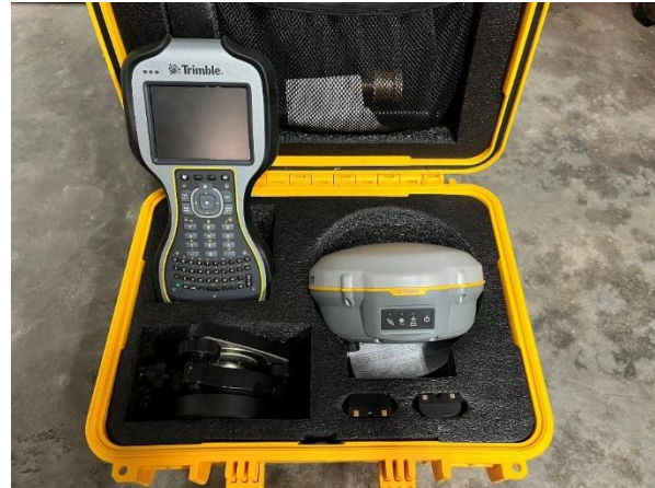
Figure 7 GNSS receiver Trimble R8s and supporting accessories
