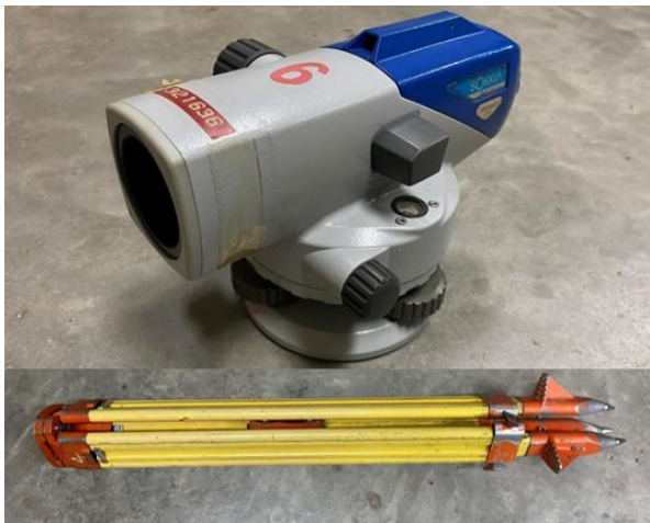
Figure 5 Leveling instrument: Sokkia C31 with tripod.
