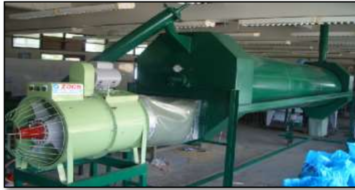
Figure 4 Rotating paddle type concurrent flow hot air paddy dryer for community level
