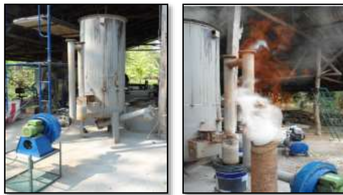
Figure 5 Design and test of the gasifier with rice husk as a fuel for drying paddy for community rice mill.
