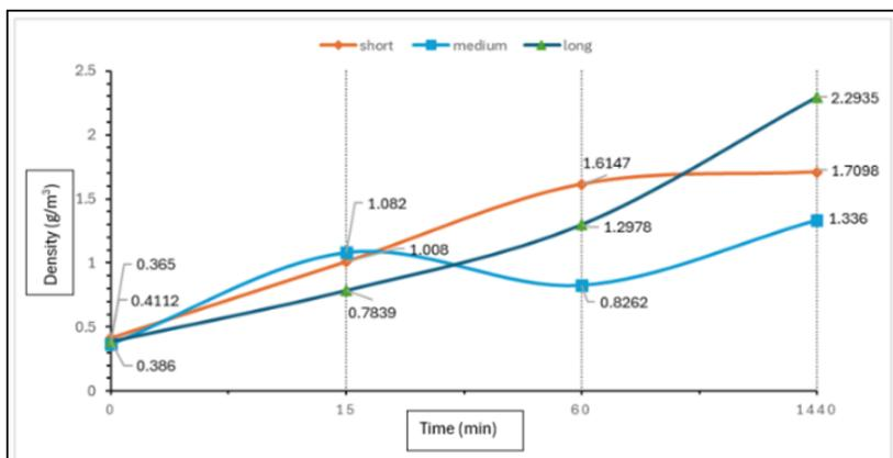
Figure 4. Change of Density after soaked in water for 15 min, 60 min and 1 day
