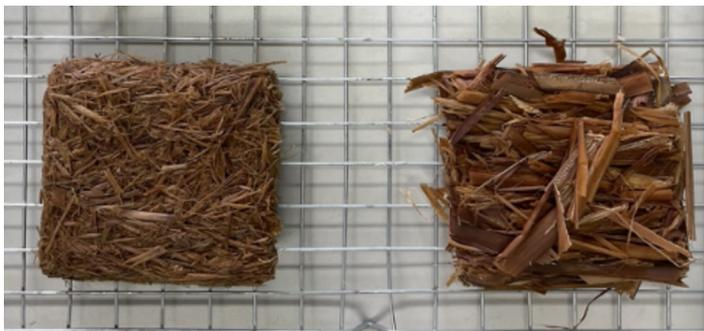
**Figure 7.** Typha thermal insulation sheet after soaked
