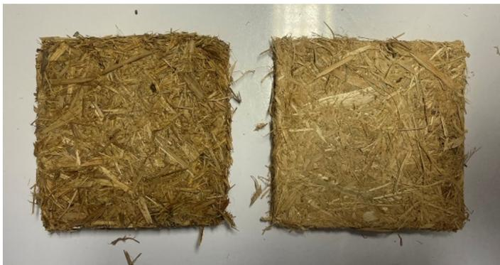
**Figure 6.** Typha thermal insulation sheet
