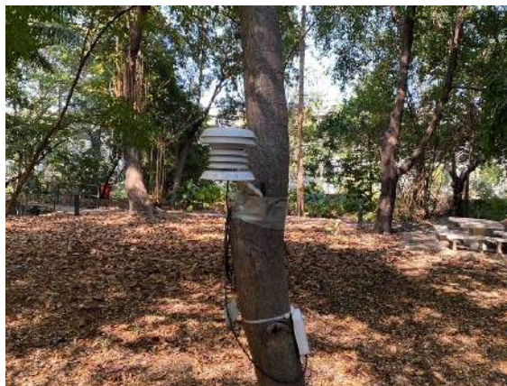
Figure 1. The Fix Station (HOBO) Temperature Sensor at the Kasetsart University, Bangkok
