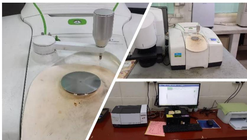
**Figure 3** ATR-FTIR setup for the analysis
