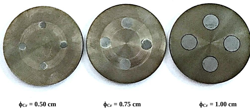
Figure 2 Position and diameters of Cr inserts in Ti target: (A) three inserts and (B) four inserts.
