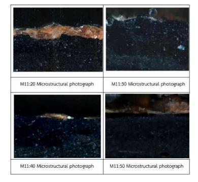
Structure of lacquer ceramic sample by using a microscope
