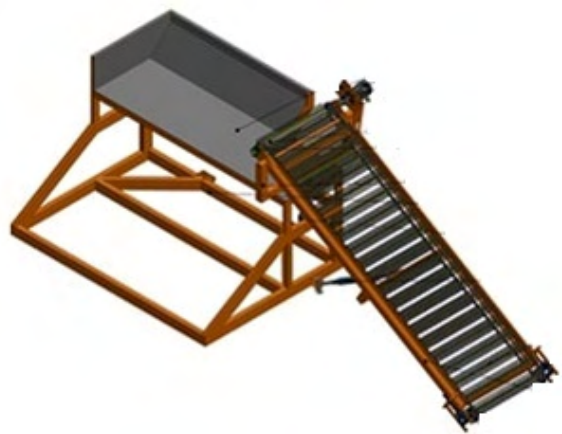
Figure 1 Cassava-root cluster conveyor drawing
