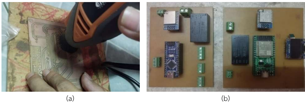
Figure 12. Drilling holes in the PCB (a), component installation on the PCB (b).
