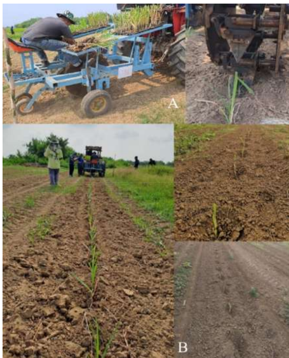
Figure 6 (A) Testing the sugarcane transplanter (B) Sugarcane seedlings after the test
