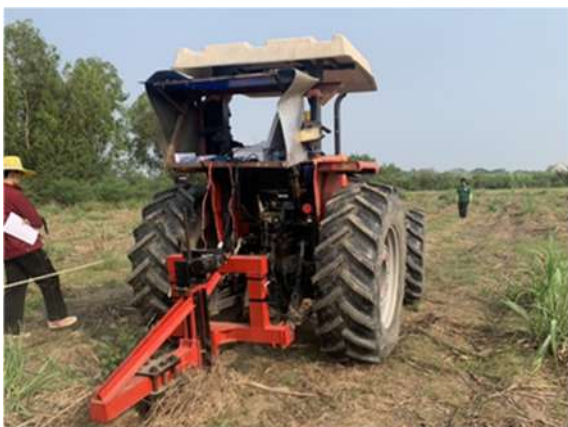
Figure 4 Automatic depth adjusting subsoiler in field testing
