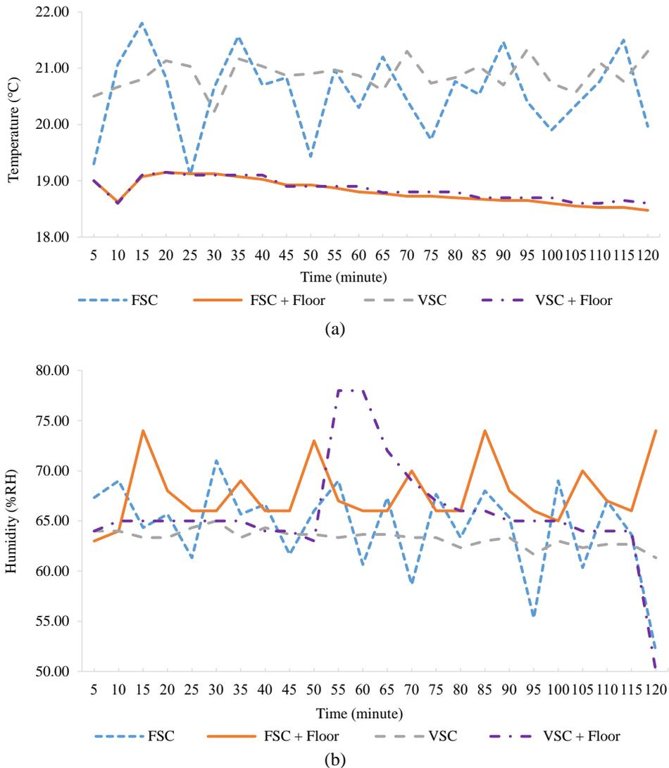
**Fig. 4.** Room (a) temperatures and (b) relative humidity provided by FSC, VSC, radiant floor cooling, and combined systems in the no-heat-load rooms; the vapor compression systems set at 22°C.
