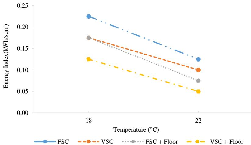
**Fig. 10.** Average energy index varied with the set temperatures of the vapor compression system obtained from FSC, VSC and combined systems in the heat loaded rooms.
