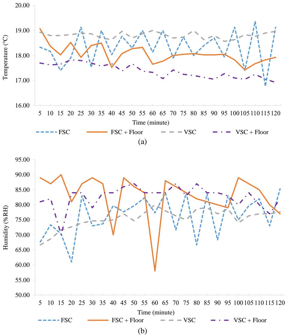
**Fig. 7.** Room (a) temperatures and (b) relative humidity provided by FSC, VSC, radiant floor cooling, and combined systems in the no-heat-load rooms; the vapor compression systems set at 18°C.
