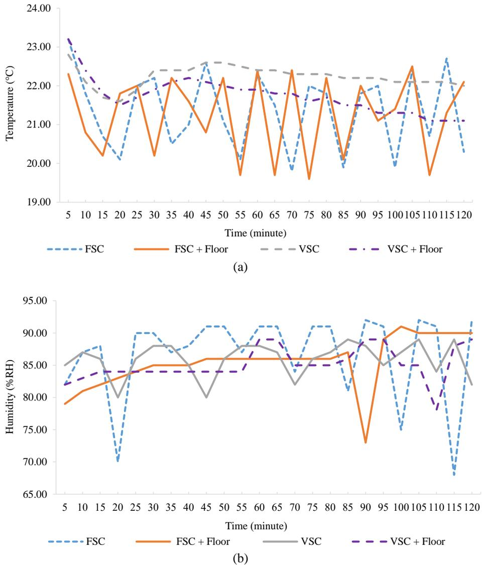
**Fig. 5.** Room (a) temperatures and (b) relative humidity provided by FSC, VSC, radiant floor cooling, and combined system in the heat loaded rooms; the vapor compression systems set at 22°C.
