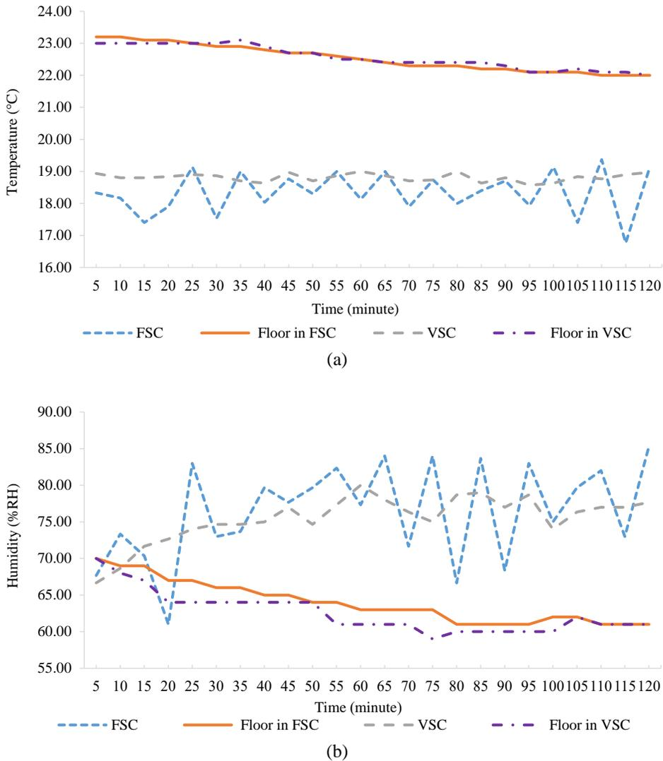
**Fig. 6.** Room (a) temperatures and (b) relative humidity provided by FSC, VSC, and radiant floor cooling systems in the no-heat-load rooms; the vapor compression systems set at 18°C.
