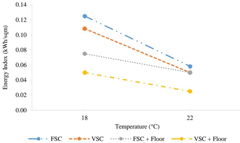
**Fig. 9.** Average energy index varied with the set temperatures of the vapor compression systems obtained from FSC, VSC, and combined systems in the no-heat-load rooms.
