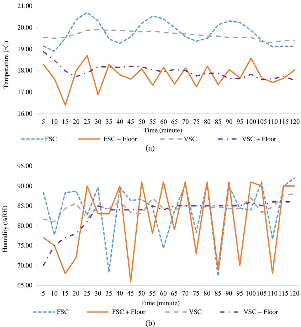
**Fig. 8.** Room (a) temperatures and (b) relative humidity provided by FSC, VSC, radiant floor cooling, and combined systems in the heat loaded rooms; the vapor compression systems set at 18°C.
