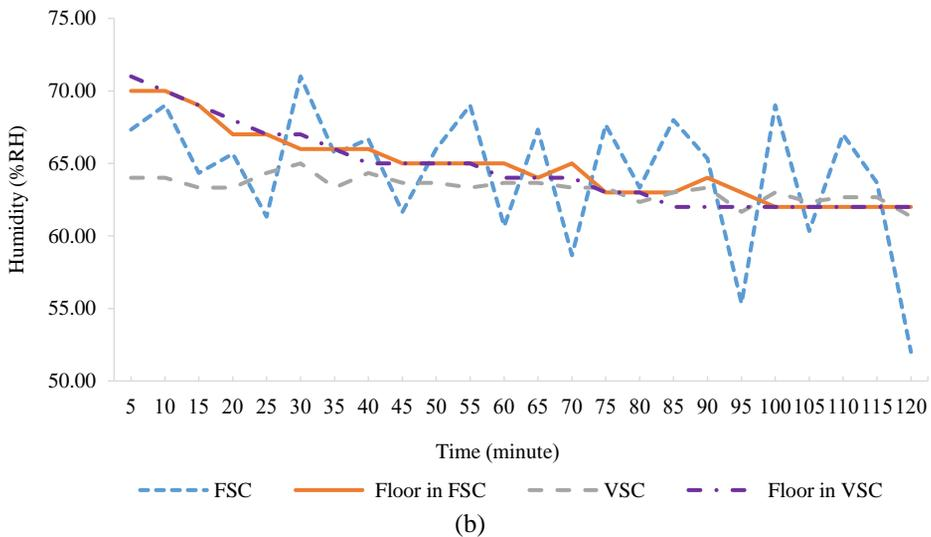
**Fig. 3.** Room (a) temperatures and (b) relative humidity provided by FSC, VSC, and radiant floor cooling systems in the no-heat-load rooms; the vapor compression systems set at 22°C.
