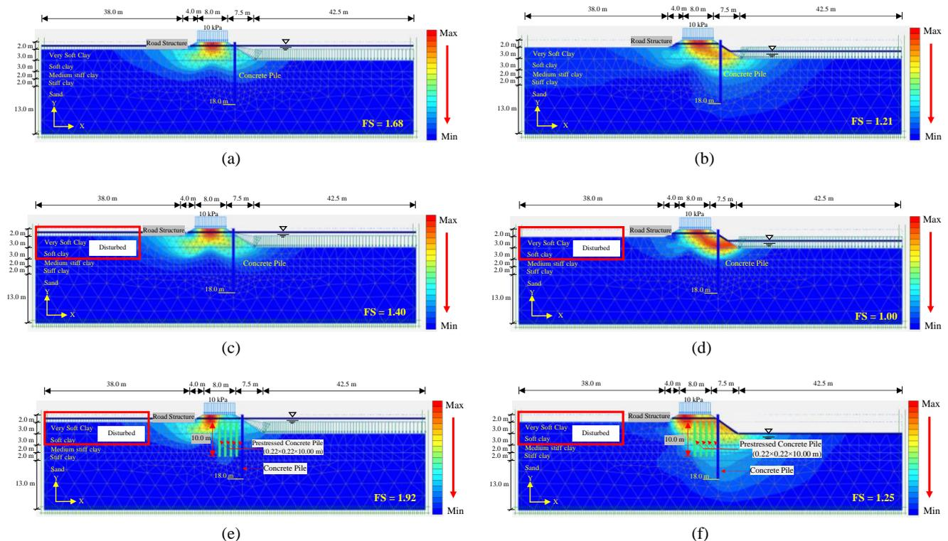
**Figure 11 Displacement contour (a) the soft clay layer under full water level (b) the soft clay layer under the water level of 3.5 m depth below the ground surface (c) the soft sensitive clay layer under full water level (d) the soft sensitive clay layer under the water level of 3.5 m depth below the ground surface (e) the reinforced by 4-row piles under full water level (f) the reinforced by 4-row piles under the water level of 5 m depth below the ground surface**
