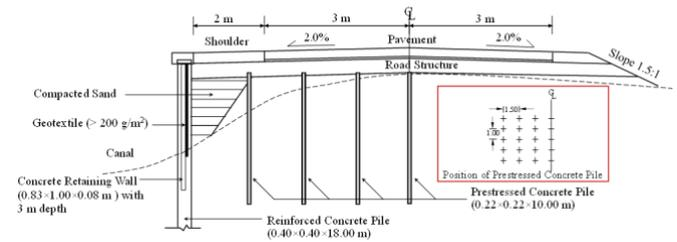
**Figure 12 Cross section of a road structure reinforced by 4-row piles**
