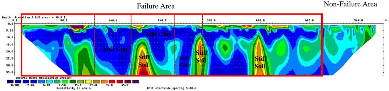
Figure 6 Resistivity survey (modified from Suksawat et al., 2023)
