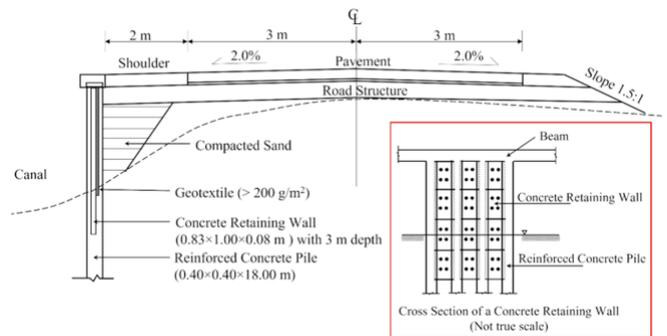
Figure 3 Cross section of a reinforced concrete pile (Suksawat et al., 2023)
