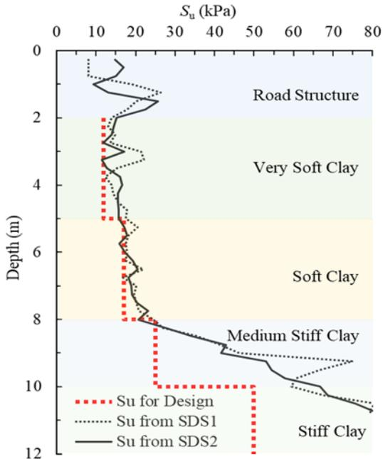
Figure 7 SDS at failure area (Suksawat et al., 2023)
