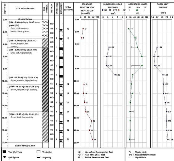
Figure 2 Boring log of NB. 5036 (Suksawat et al., 2023)
