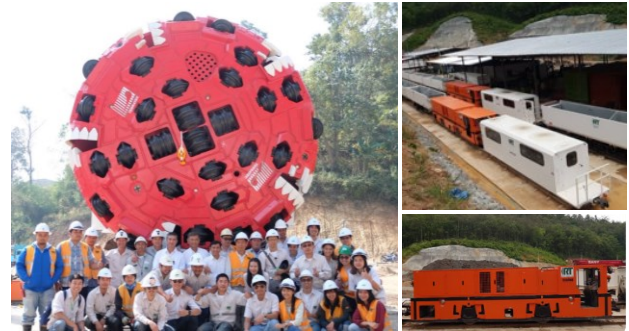
Figure 5 Illustrate T57 double shield TBM and rolling stock fleets
