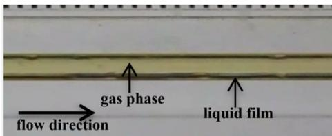
**Fig. 5.** Annular flow ( $J_G = 36.964$  m/s,  $J_L = 0.091$  m/s).
