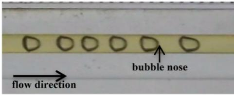
**Fig. 3.** Bubbly flow ( $J_G = 0.207$  m/s,  $J_L = 0.879$  m/s).
