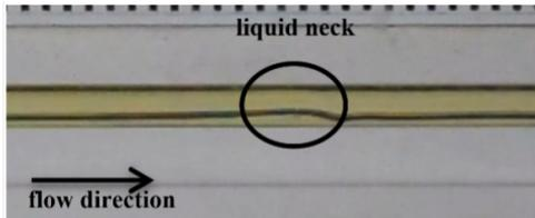
**Fig. 4.** Plug-annular flow ( $J_G = 1.941$  m/s,  $J_L = 0.033$  m/s).
