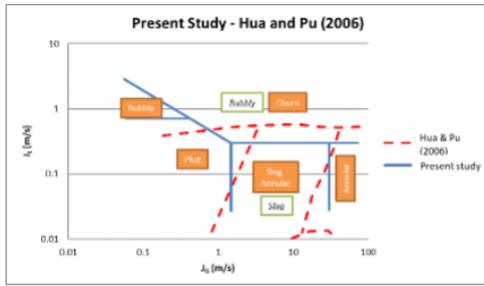
**Fig. 11.** Flow pattern map comparison of the current study and by Hua and Pu [23].
