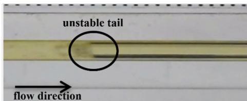
**Fig. 6.** Churn flow ( $J_G = 0.207$  m/s,  $J_L = 2.297$  m/s).
