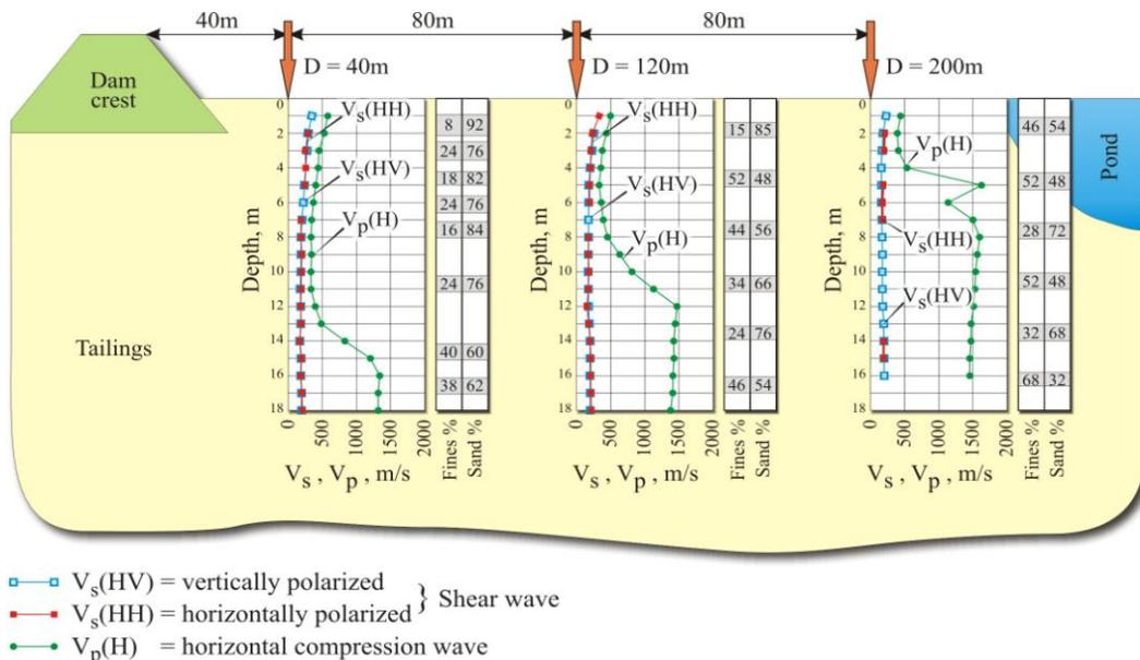
Figure 15. West Dam, cross-hole tests results
