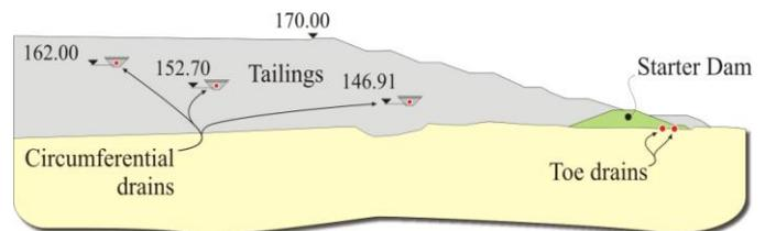
Figure 6. East Dam, location of the circumferential drains
