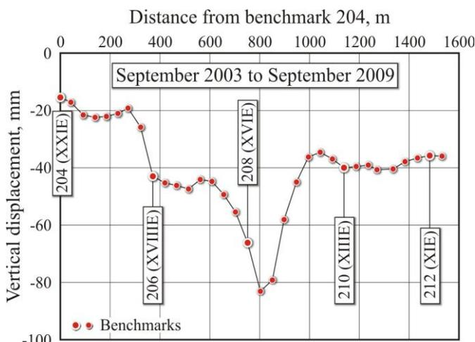
Figure 23. East Dam, vertical displacement along the crest of the starter dam
