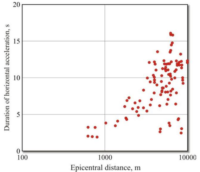
Figure 20. Duration of shaking vs. epicentral distance
