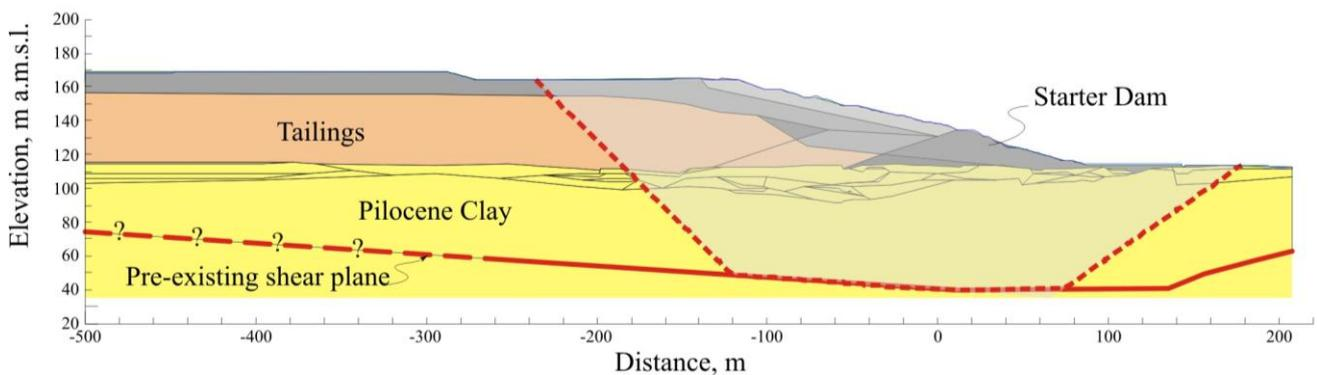
Figure 25. East Dam, cross-section XVI-E, critical failure body
