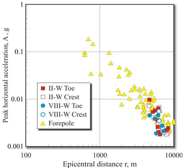
Figure 19. Peak ground acceleration vs. epicentral distance
