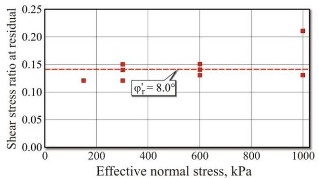
Figure 10. Ring shear residual strength
