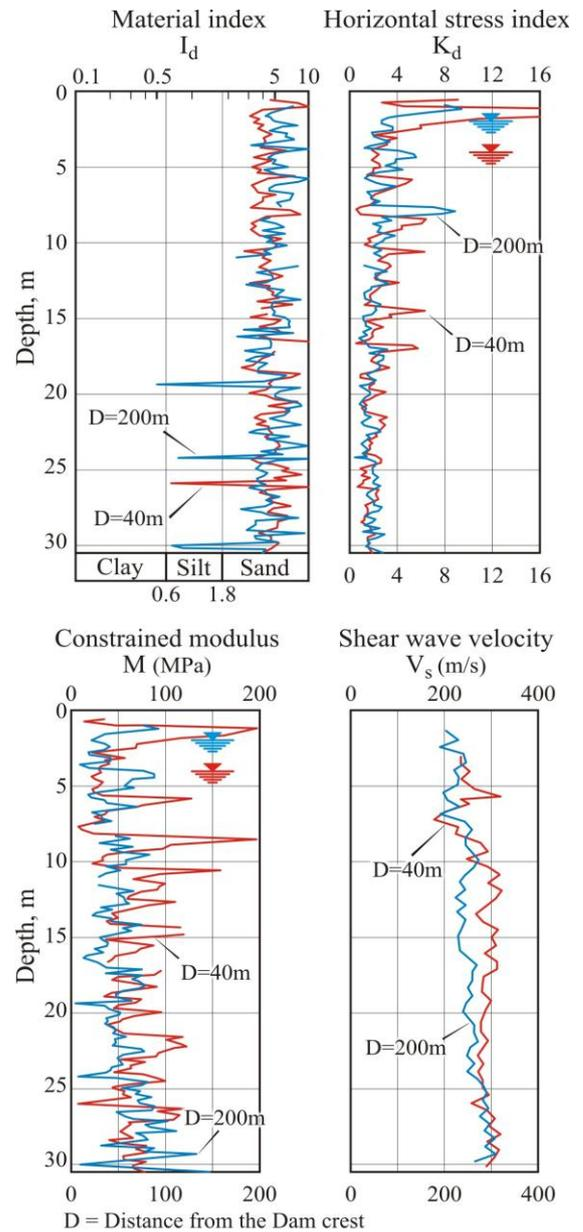
Figure 13. East Dam, results of two S-DMT's
