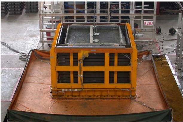
Figure 7. Mailiao sand specimen in the shear box on shaking table
