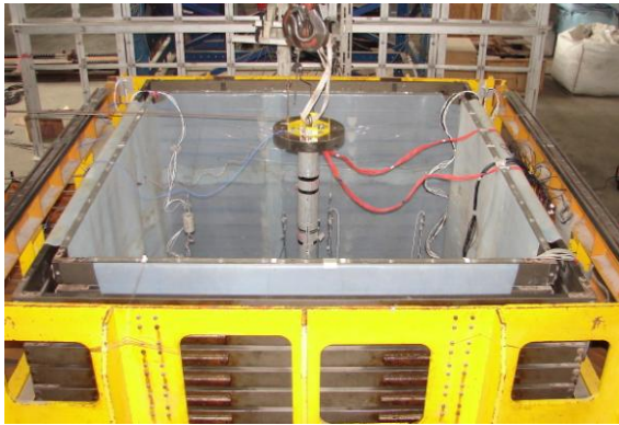
Figure 4 The instrumented aluminum pipe inside the shear box with one steel disk on the top
