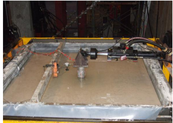
Figure 8. Lateral load test on the steel model pile
