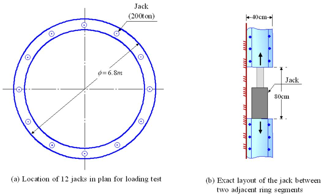
(a) Location of 12 jacks in plan for loading test
