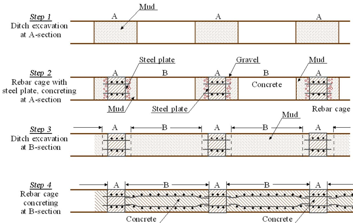
Figure 39 Diaphragm wall by rebar lapping method
