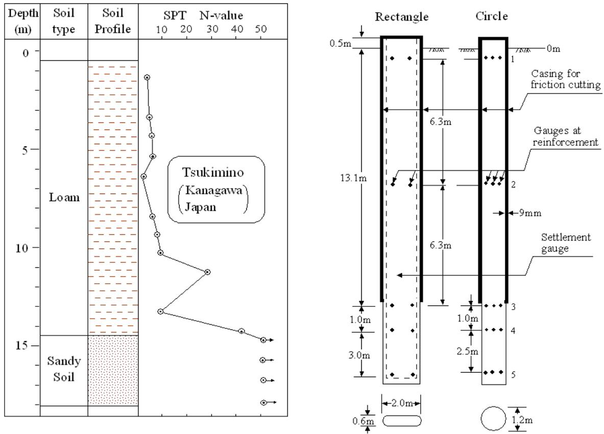
Figure 17 Soil profile and side view of the two piles (Iwanaga et al. 1991)
