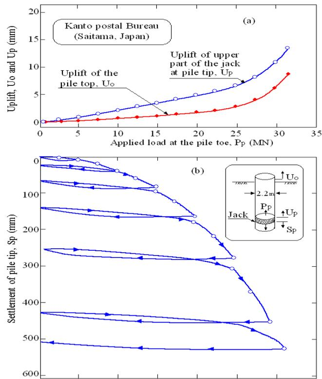
Figure 4 Results of the pile toe loading test at the site of Kanto Postal Bureau (Shibuya et al. 1997)
