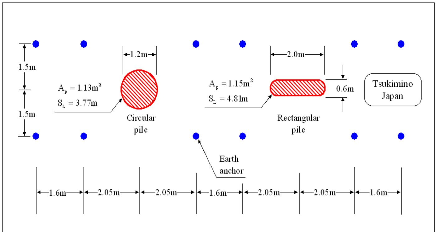
Figure 16 Layout of the pile loading tests, one on a circular and the other on a rectangular pile at Tsukimino (Iwanaga et al. 1991)
