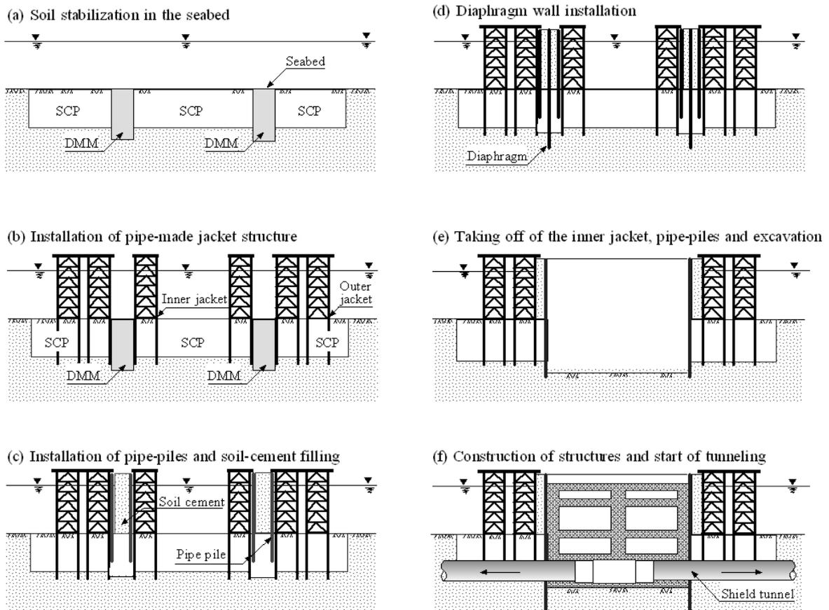
Figure 46 Construction process of the man made Island
