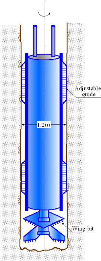
Figure 41 Cutting machine for the ditch
