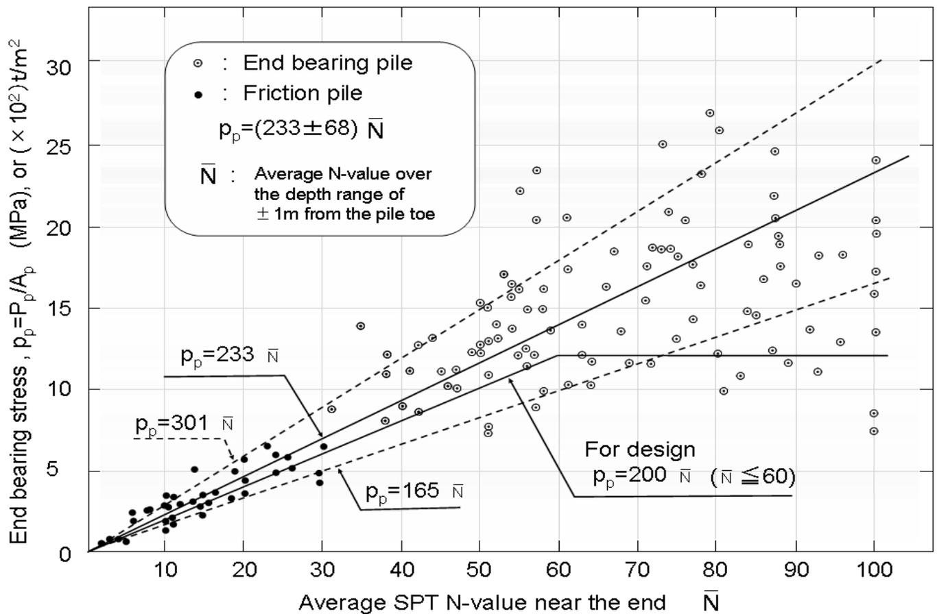
Figure 32 Summary plots of the ultimate toe bearing load intensity as function of averaged N-value (from Japanese manual)
