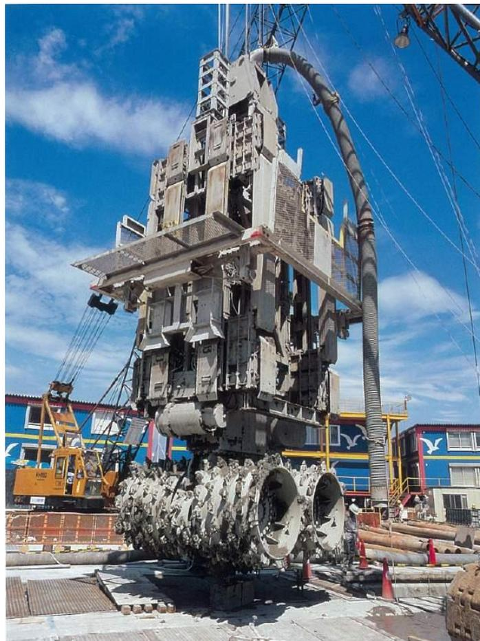
Figure 49 Two-axes rotating type cutting bits
