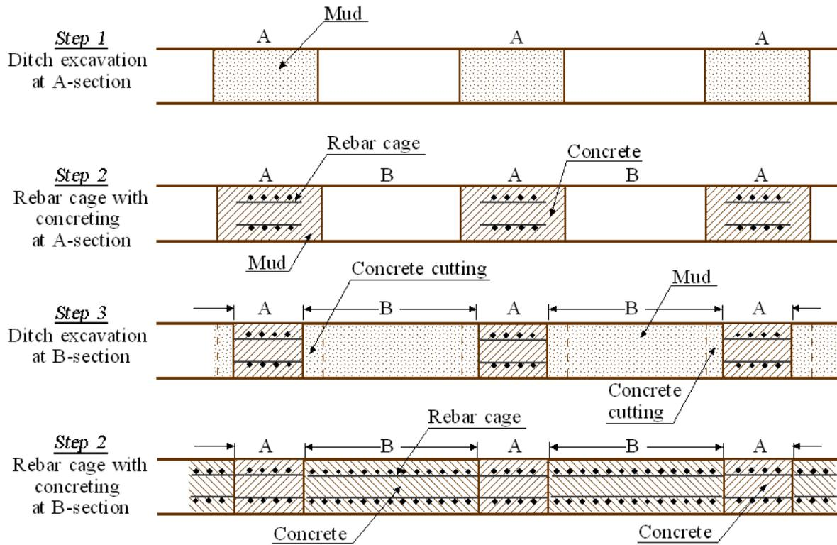
Figure 40 Diaphragm wall by concrete cutting method
