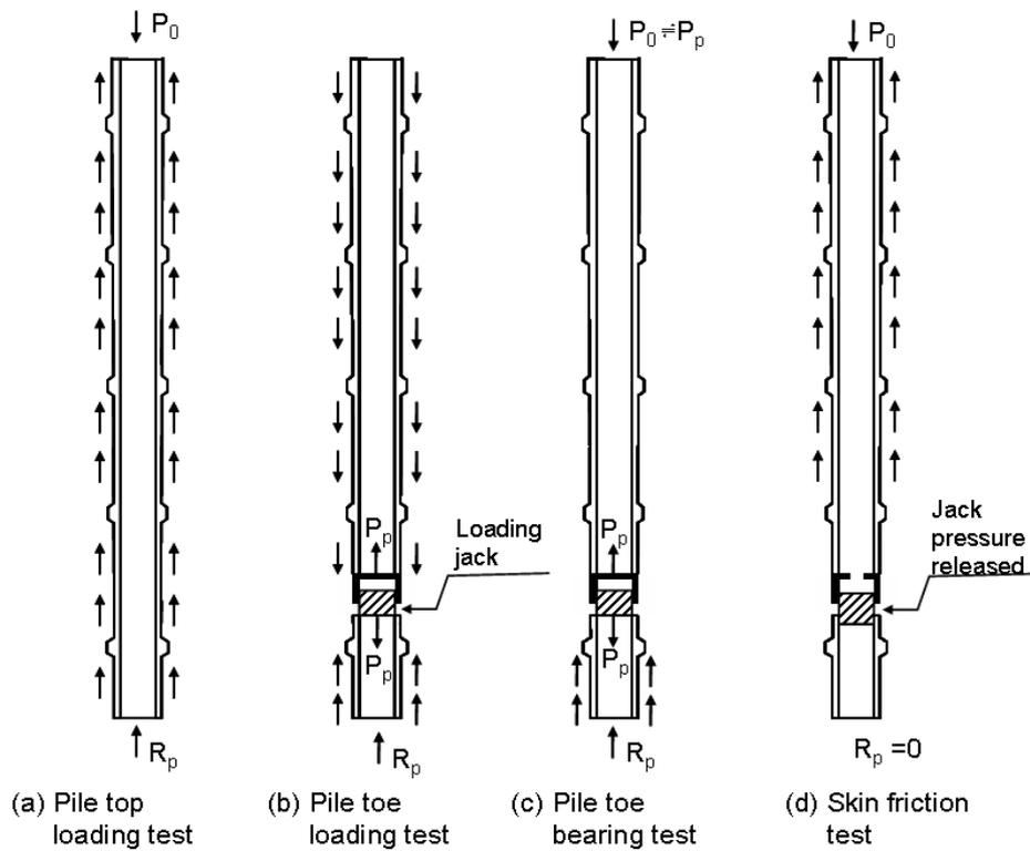
Figure 9 Four types of pile loading test
