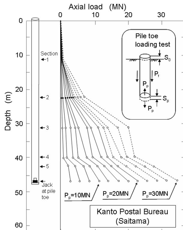
Figure 5 Axial load versus depth in the pile toe loading test at Kanto Postal Bureau (Shibuya et al. 1997)
